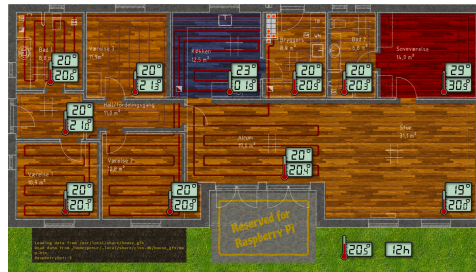
Fig. 3. Digital twin of a floor heating system
