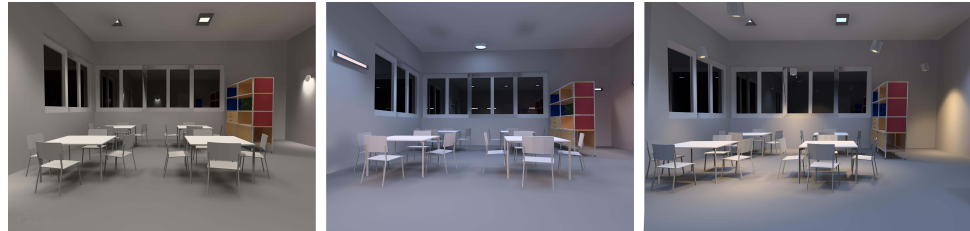
Figure 13. Shadow qualities of the three options. The various combinations of lighting fixtures result in either diffused or sharper shadows.
