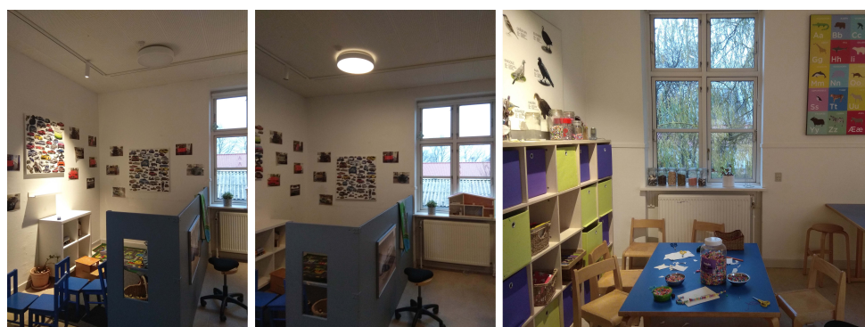
Figure 10. Vuggestuen Tummelumsen, Roskilde visit, photo registration. As seen for the left, in the first photo, only the recently installed spotlights are turned on. In the second photo, the ceiling light is on. In the third and last photo, the spotlights are on highlighting the wall and complementing the daylight coming from the window. Personal archive.
