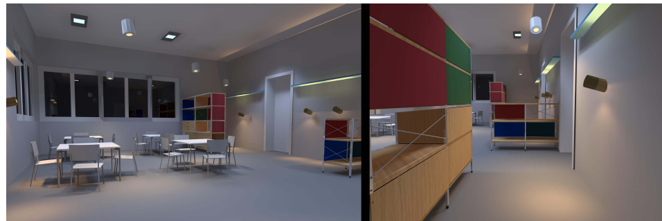
Figure 15. Shadows and the use of reflectors in classroom. The light fixtures in these renderings have both an upwards and downwards distribution. The horizontal reflectors in the classroom redistribute the upward lighting coming from the wall fixtures.
