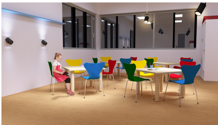
Figure 19. Illustration of the proposed lighting strategy. The rendered image is used to illustrate the topology of each fixture and the shadows in the space.
