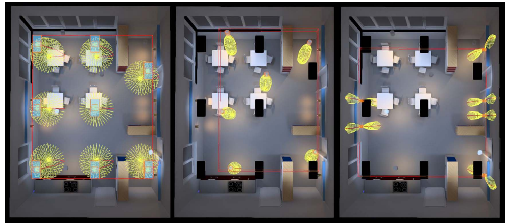
Figure 14. The light distributions of the different fixtures. As seen from the left, the first rendering depicts the ceiling lights that have a wider distribution. The middle rendering illustrates the spotlights with a narrow light distribution. In the last rendering, the wall light distribution can be seen.
