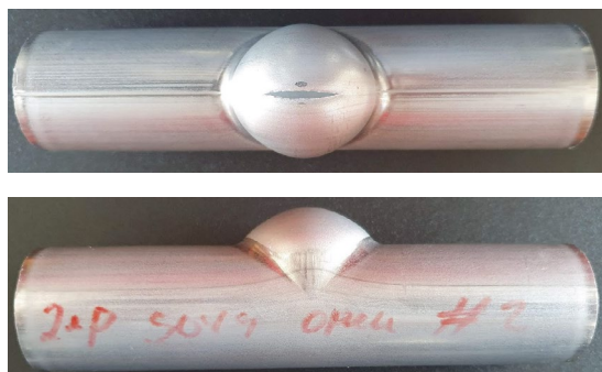
Fig. 8 Results from the bursting experiment (double the forming pressure), where the feedback system stabilizes the process by reducing the pressure (material 5049-O)
