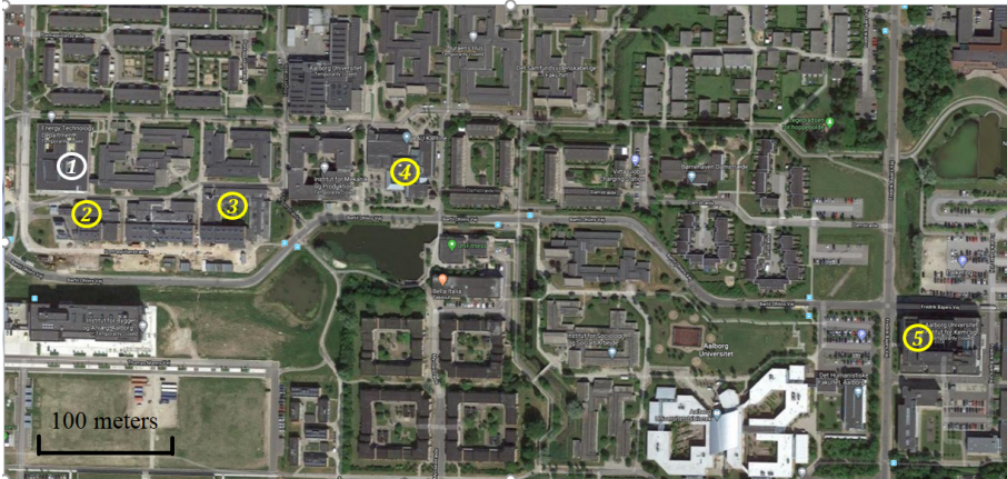
Fig. 4.6: LoRa coverage field test layout. Payload size: twenty bytes - Image source:Google Maps, Aalborg University campus.
