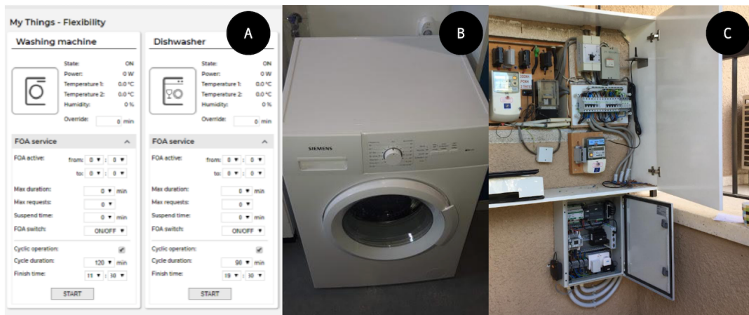
Fig. 1. GOFLEX project household HEMS technology: A) An English version of a user interface to control flexibility parameters from the Cyprus demonstration site. B) A washing machine controlled by a smart plug at the German demonstration site. C) HEMS technology installed next to the meter cabinet in a household in Cyprus.
