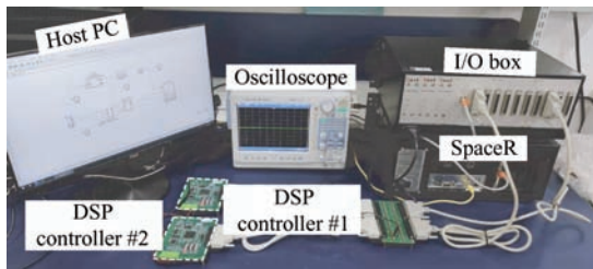
Fig. 2 Photo of the HIL experimental setup
