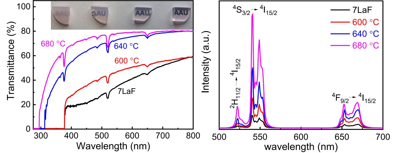
Light transmittance and UC Luminescence:
