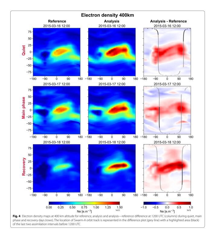
line) with a highlighted area (black) representing the last two assimilation windows (20 min) of the satellite's path before 1200 UTC. The effect of the assimilation at different altitudes extends in a range from 200 km to 1000 km, finding the maximum differences between reference and analysis at mid-low latitudes around the assimilation altitude from 200 to 600 km (not shown here).
