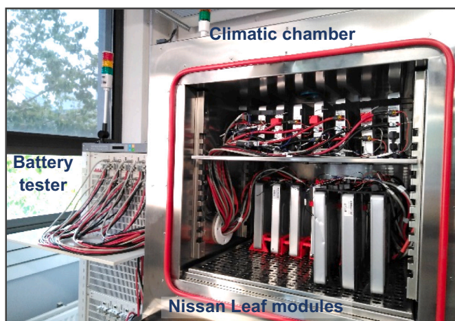
Fig. 1. Example of Nissan Leaf modules under test and experimental test bench.
