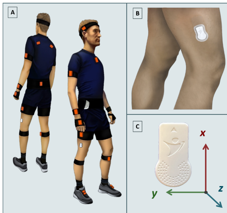
Figure 1. (A) Simultaneous application of SENS and Xsens sensors (Xsens sensors are shown on top of clothing for illustrative purposes). (B) Placement of a SENS sensor on the distal lateral side of the thigh. (C) Coordinate axes of the SENS sensor.
