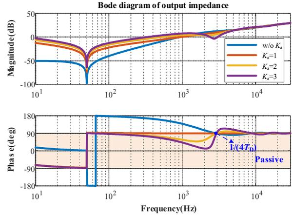
Fig. 3. Bode diagram of output impedance under various  $K_a$ .
