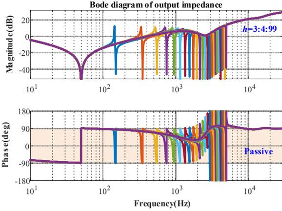
Fig. 4. Bode diagram of output impedance ( $N_c=5$ ).
