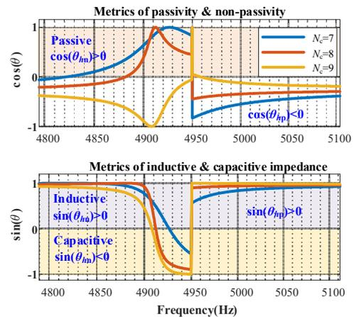
Fig. 7. Impact of  $N_c$  on modified passivity metrics under  $h=99$ .
