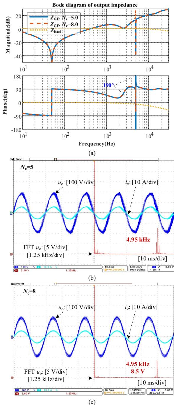
Fig. 14. Bode diagram of output impedance and experimental results of Case III (Stage 4).  $h=99$ ,  $R_{load}=32 \Omega$ ,  $C_{load}=0.2 \mu\text{F}$ . (a) Bode diagram. (b)  $N_c=5$ . (c)  $N_c=8$ .
