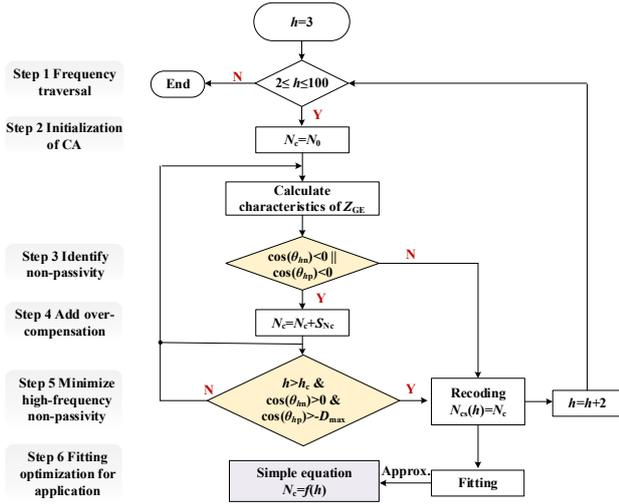
Fig. 8. CA design based on the constrained piecewise linear fitting.
