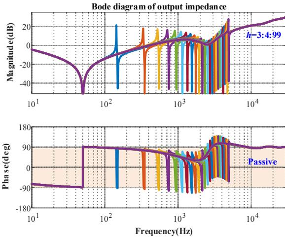
Fig. 5. Bode diagram of output impedance ( $N_c=8$ ).
