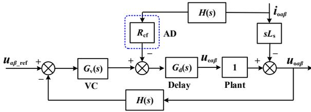
Fig. 2. Control diagram of the single-loop voltage control with AD.
