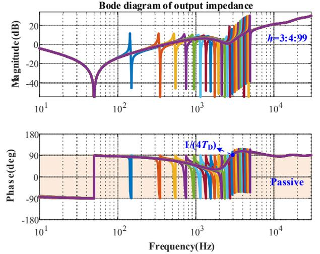
Fig. 10. Bode diagram of output impedance (Presented  $N_c$ ).
