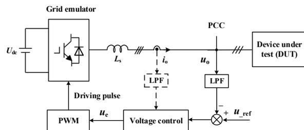
Fig. 1. General diagram of the grid emulation system.
