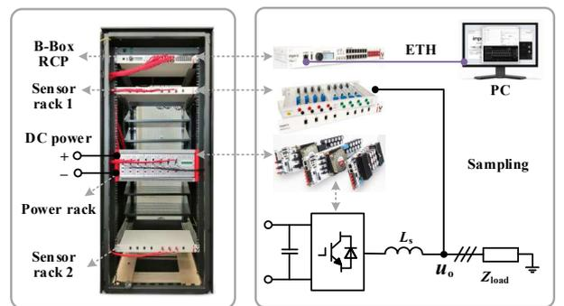
Fig. 11. Experimental setup of three-phase PWM inverter with  $L$  filter.
