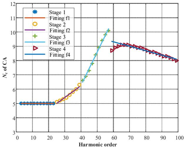
Fig. 9. The first-order piecewise fitting between  $N_c$  and  $h$ .
