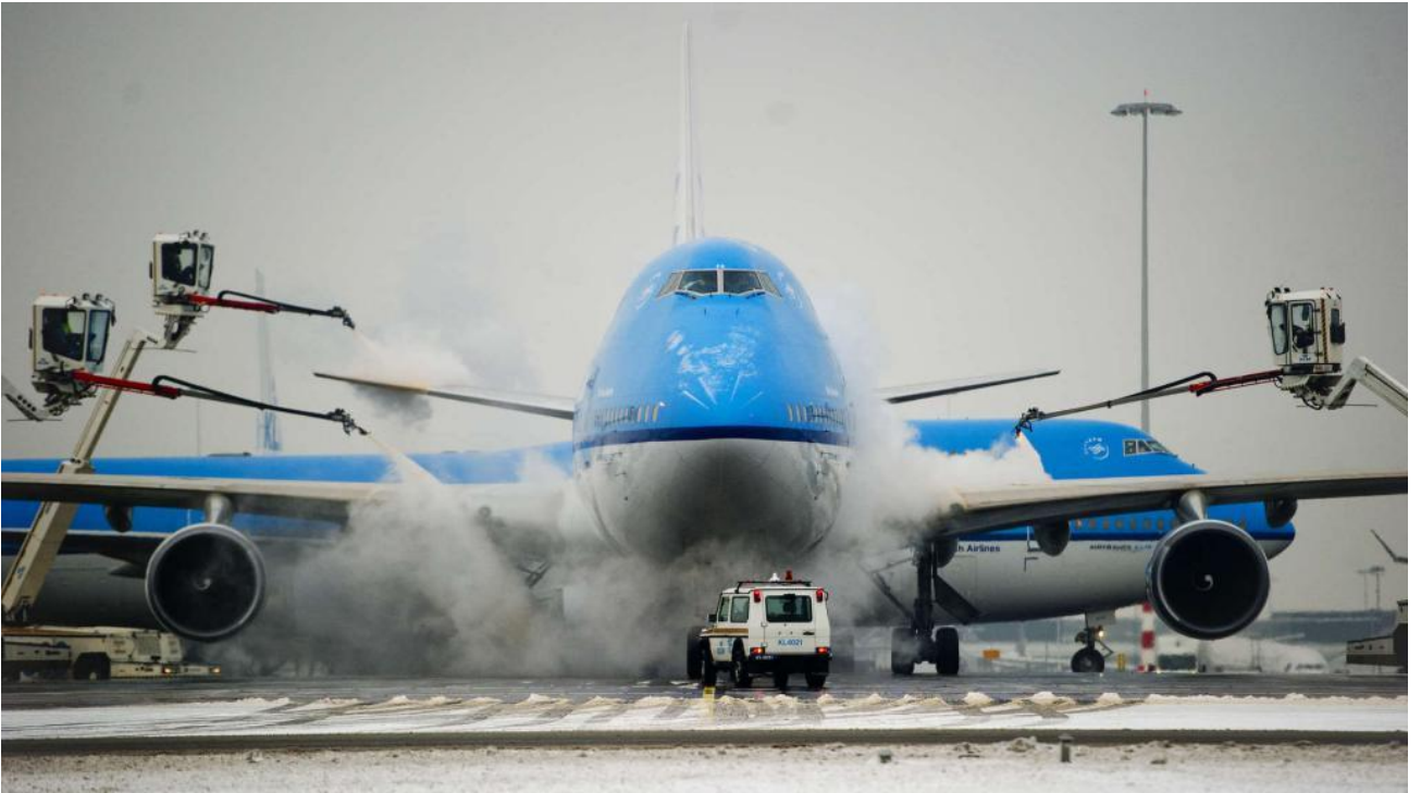
Fig. 4.4 - Aircraft treatment with type I anti-icing liquid
