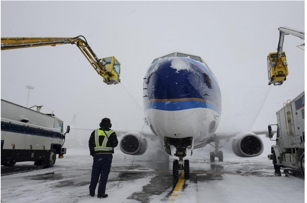
Fig. 4.5 - Aircraft treatment with type IV anti-icing fluid
