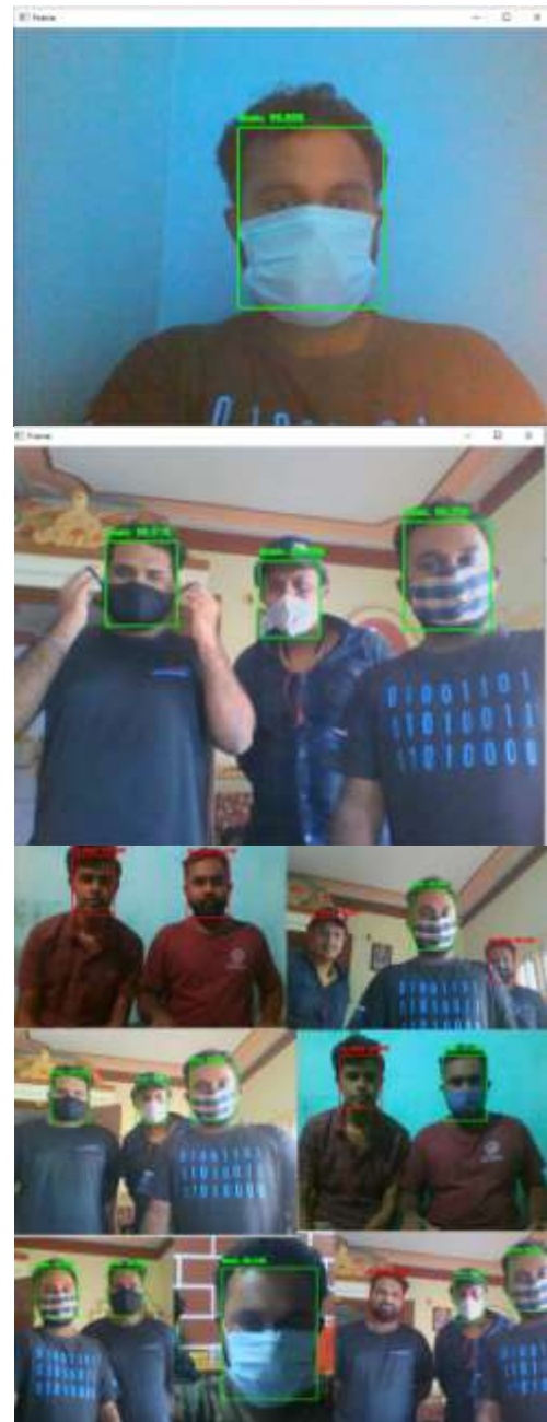
Fig 4: The results for no mask and wearing mask. As in the Figure 4, it can be clearly seen that the green box indicates the inclusion of the mask whereas the absence of mask is indicated as red color.
