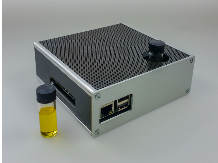
Figure 1. Photo of the fluorescence sensor and olive oil samples in the glass vials.
