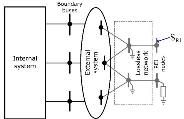
Fig. 4. Inclusion of the lossless network and REI nodes.
