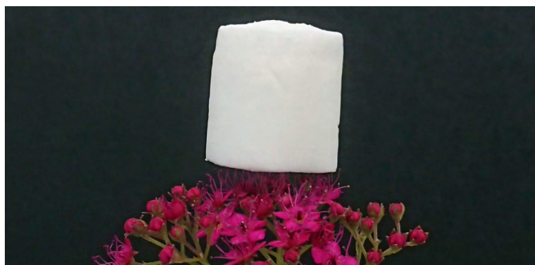
Ultralight chitosan nanofiber sponge supported by the pistils of a steeplebush ( Spiraea ) (Reprinted with permission from DOI: 10.1021/acsapm.1c00799 Copyright 2021 American Chemical Society.)
