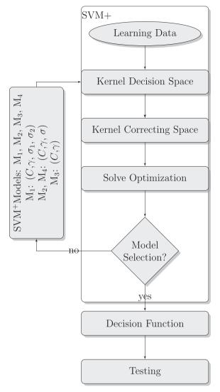
**Fig. 2.** SVM+ learning diagram model. Models M<sub>1</sub>, M<sub>2</sub>, M<sub>3</sub> and M<sub>4</sub> are selected according to the kernels parameters for the decision space and the correcting space.
