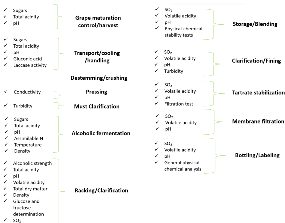
Figure 2. The most important steps of classical white winemaking with the identification of the most common analytical determinations.
