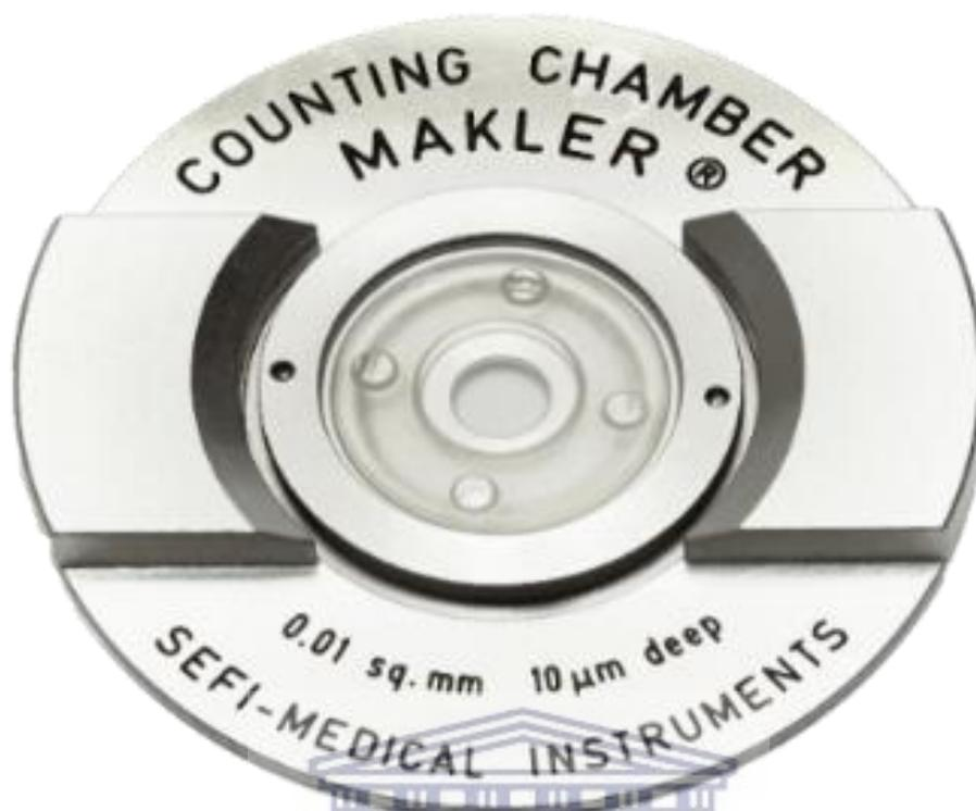
Figure 2.1: Makler counting chamber used for to determine sperm concentration
