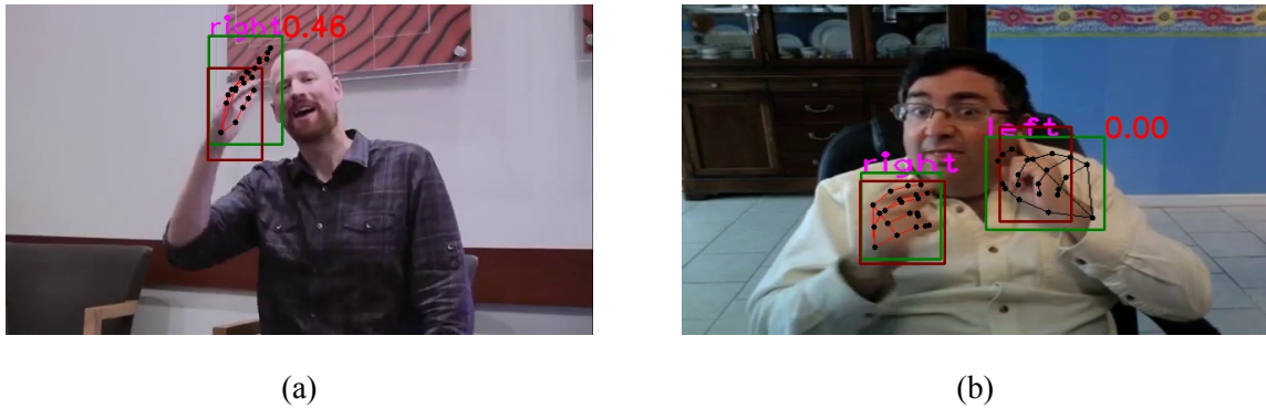
Figure 4.2: Cases of false positives with a low IoU (a) and false hand classification (b)
