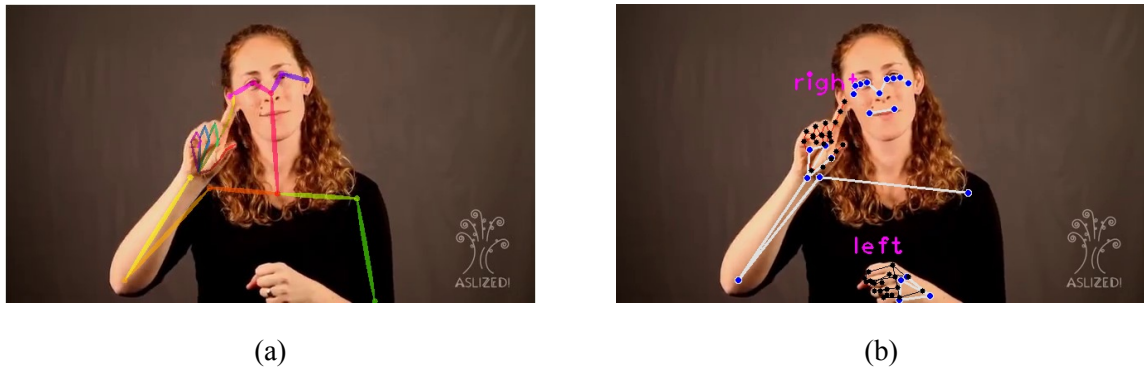
Figure 3.1: Examples of generated keypoints on a sample frame of the ChicagoFSWild dataset, employing (a) OpenPose and (b) MediaPipe
