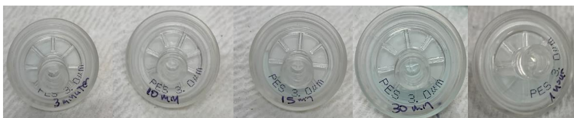
Figure 61. Visual representation of the effect of incubation time on detection signal. From left to right, the filters were incubated for 3, 10, 15, 30 and 60 minutes
