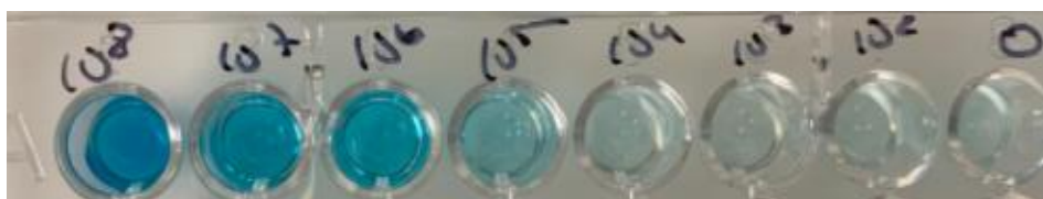
Figure 10. Visual limit of detection for formalin-inactivated Cryptosporidium using HRP-labelled antibodies. A blue color indicating the presence of oocysts is shown.
