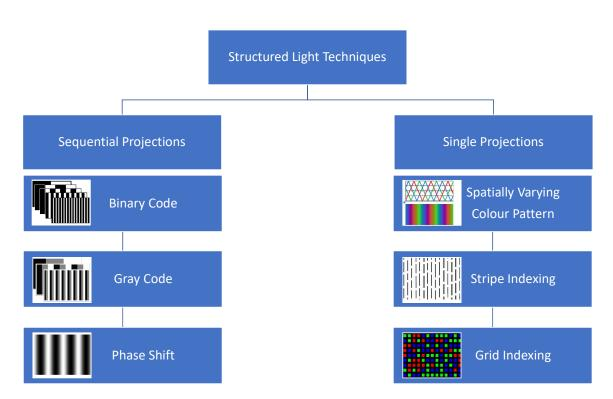
Figure 2.4: Illustration of different structured light methods categorized by sequential images versus single images projected and captured. Example images copied from [19].
