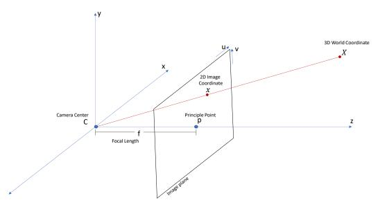
Figure 2.1: The pinhole camera geometry model relates a 2D coordinate x in an image plane to a 3D observed world coordinate X through projective transformations.
