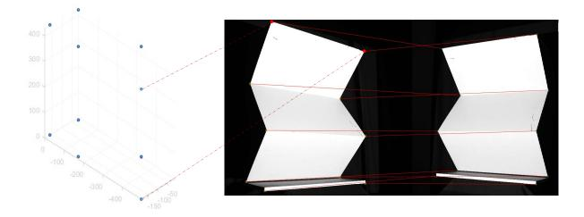
Figure 3.3: Example of a virtual calibration target. Key points of the synthetic model (left) are matched to their locations in the point correspondence sets of two moving camera views. Lines added to visualize the correspondence relationships.
