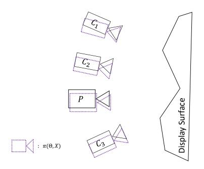
Figure 2.5: Illustration of bundle adjustment refinement. Image planes are estimated based on known or approximate 3D display surface coordinates and camera or projector calibration parameters. Estimated image planes (purple) are compared with the measured image planes (black) and the parameters used to generate the estimated image planes are adjusted to minimize the difference.
