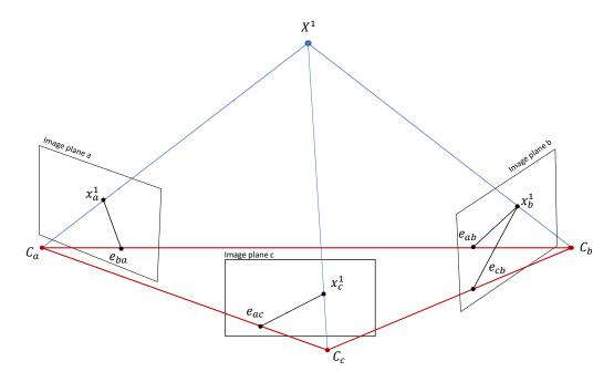
Figure 2.3: Epipolar geometry relates 2D pixel coordinates  $x_a$  in image a to the observed 3D coordinate X and the corresponding 2D pixel coordinates  $x_b, x_c$  in a second image b and a third image c.
