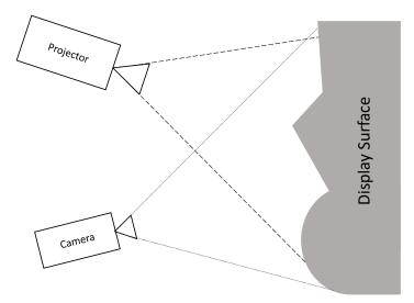
Figure 1.3: Diagram of a simple Projector-Camera System.
