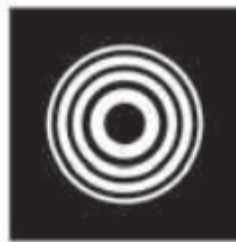
Fig. 6. An FPI interference pattern. The dark rings are for destructive interference and the light ones are for constructive interference.
