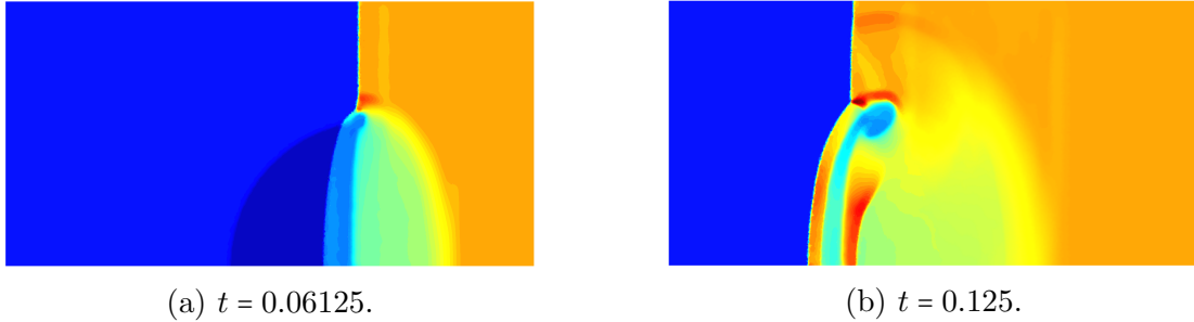
Figure 9.8: Density profile along z = 0.02 for the bubble shock interaction case using p = 1 DG approximation on an unstructured mesh of 11,530,455 tetrahedra.
