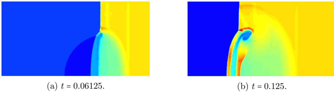
Figure 8.7: Density profile along z = 0 for the bubble shock interaction case on an unstructured mesh of 11,530,455 tetrahedra.
