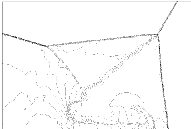
Figure 5.13: Density isolines at t = 0.2 for the double Mach test case for p = 1 with moment limiter on a final mesh of 230,266 quads.
