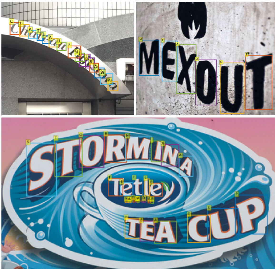
Figure 7.2: Qualitative results of the proposed method in out of distribution samples from Total-text [72] and CTW-1500 [86] datasets. The proposed method detects characters in arbitrary-shape text instances. The above images are from the mentioned public benchmark datasets [72, 86].
