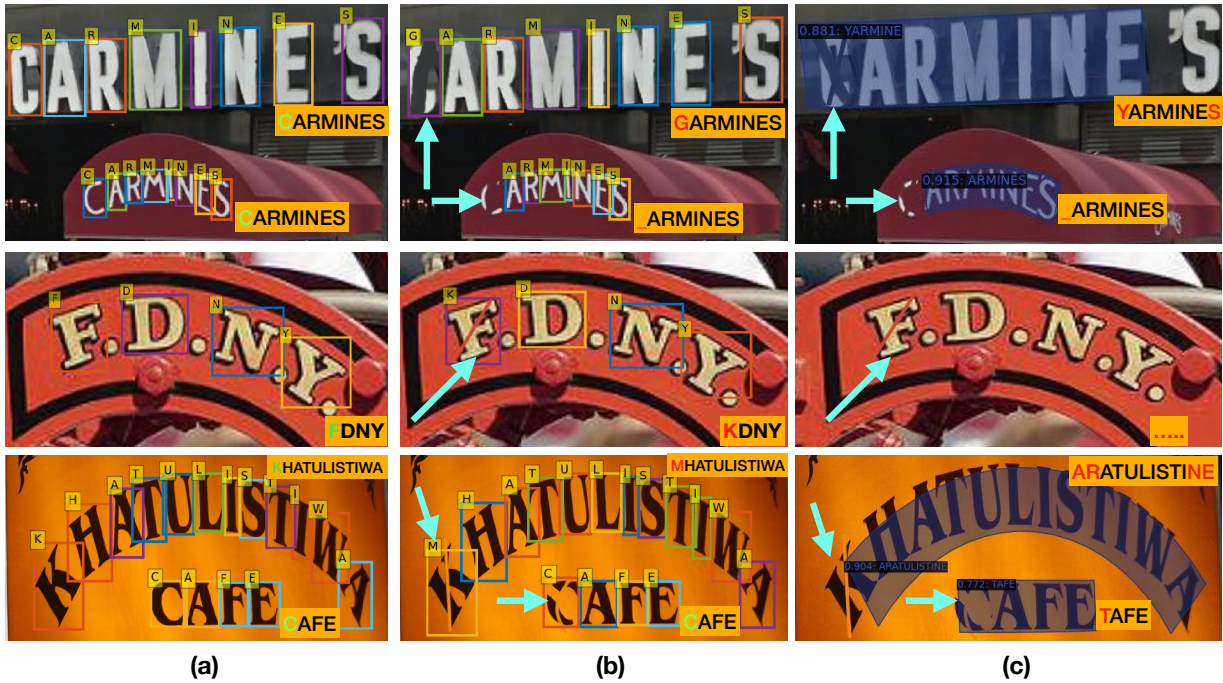
Figure 8.2: Comparison of the effect of partially occluded characters on the state of the art end-to-end scene text spotting models on some sample of Total-Text dataset [72]; results of character-based text spotting model [250] in (a) without occlusion and (b) with occlusion, and (c) shows results of [100] on occluded text instances. The “cyan” arrow, “green”, and “red” characters in yellow text denote the occluded characters, correctly recognized and missed characters by the models, respectively [We replicated these results using the pre-trained models in [100, 250]]. Best viewed in color when zoomed. The above images are taken and reproduced from the public benchmark dataset [72].
