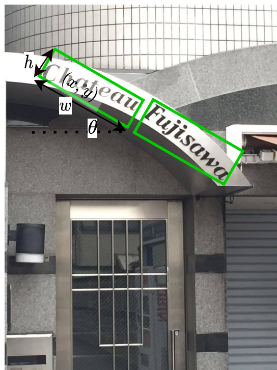
(b) Rotated Rectangle bounding box (x, y, w, h, \theta)
