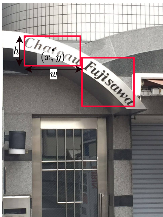
(a) Rectangle bounding box (x, y, w, h)
