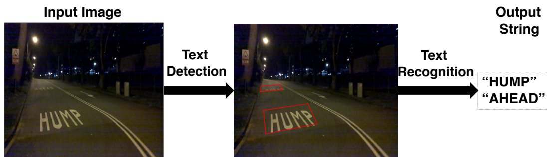
Figure 2.1: General schematic diagram of scene text detection and recognition, where sample image is from the public dataset in [119].
