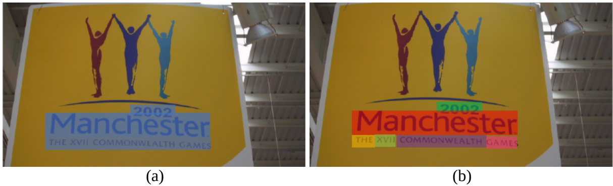
Figure 2.3: Semantic vs. instance segmentation. Ground-truth annotations for (a) semantic segmentation, where very close characters are linked together, and (b) instance segmentation. The image comes from the public dataset in [82]. Note, this figure is best viewed in color format.
