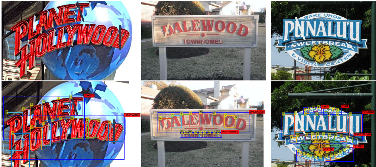
Figure 8.7: Experiment results of the proposed model that successfully spotted the occluded text instances of the occluded input images. The top images are the original images with occlusion, and the bottom are our end-to-end text spotting results (Best viewed in color when zoomed). The result character images are reproduced from publicly available benchmark dataset [72].
