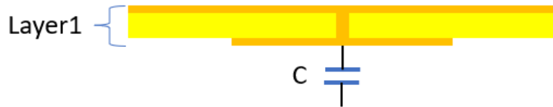
Figure 3.16: Equivalent circuit model of mechanically tunable reflectarray.
