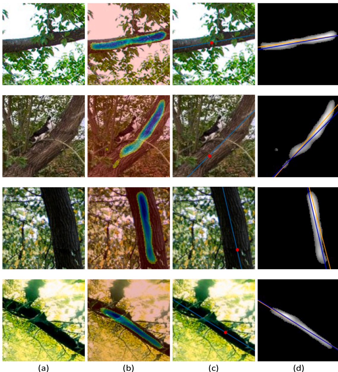
Fig. 8. Examples of the (a) original image, (b) CNN prediction, (c) Hough transform (blue line), and (d) ground truth (orange line).
