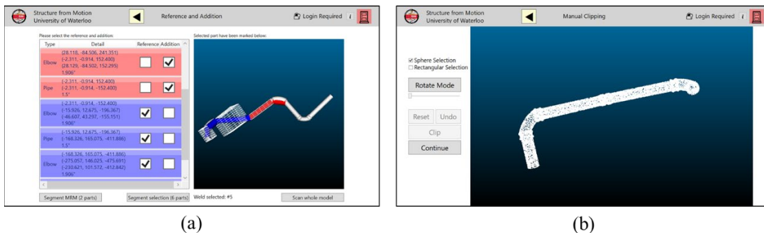
Figure 2-3. Part segmentation for assembly planning and control. (a) Referenced components are coloured in blue, and components to be added are coloured in red. (b) Segmented model point cloud automatically generated.
