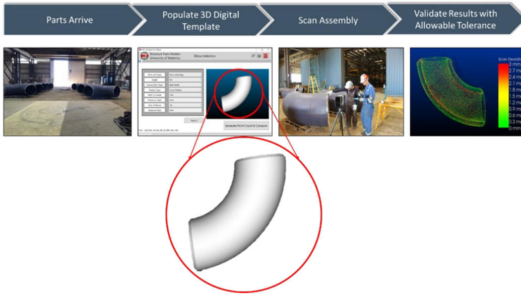
Figure 3-14. Workflow for using scan-vs-BIM at the receiving stage
