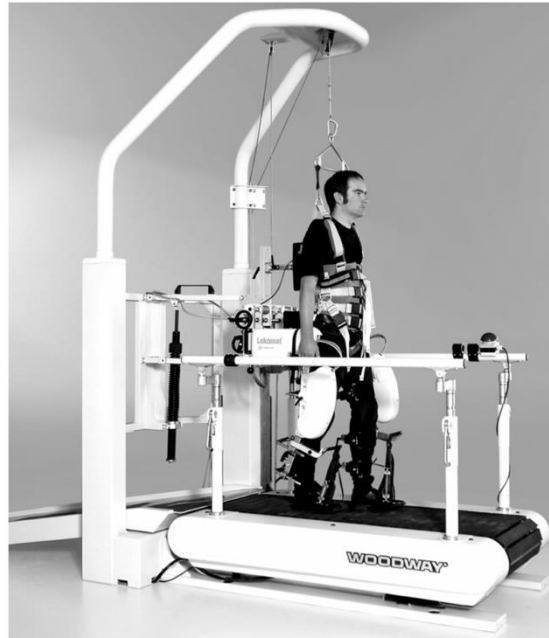
Fig. 1. The Lokomat® is a driven gait orthosis with electromechanical drives for hip and knee joint (2 degrees of freedom per leg) [1, 2]. (With permission of Hocoma AG, Volketswil, Switzerland)
