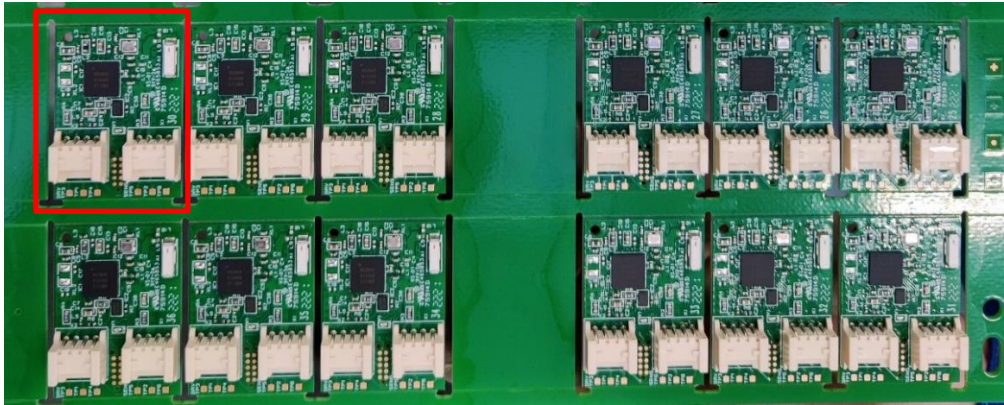
Figure 5. 12 pieces of uncut, mounted PCBs for the self-learning sensor. One PCB unit (38 mm x 18 mm) is marked in red (Photo: Lotta Marjamäki).
