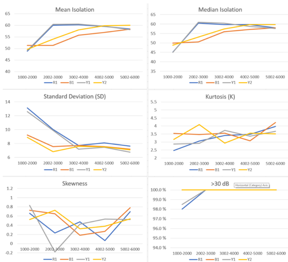
Figure 40. Statistical characteristics of CLTA B frequency subsets per antenna.
