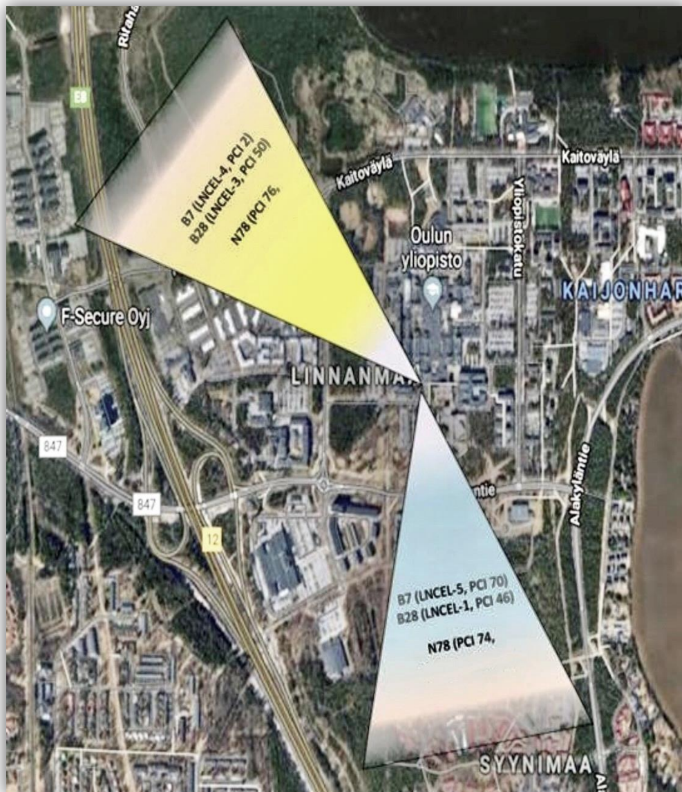
Figure 17. Anchoring information and coverage area of 5G NR in the University of Oulu.
