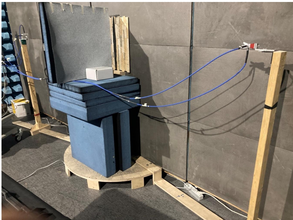
Figure 6. Photograph of dual-polarized 6 – 50 GHz measurement at wide angle measurement.
