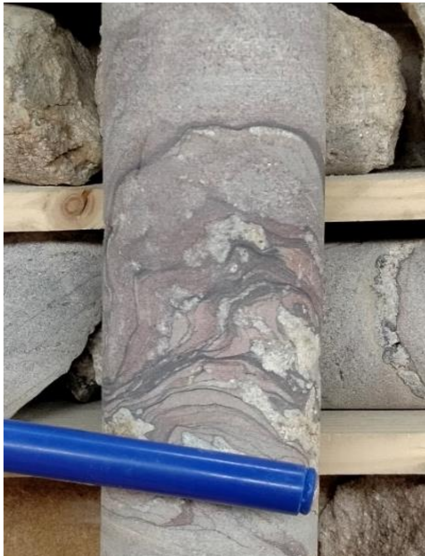
Figure 5. Photograph of drillcore showing flaser (individual mud drapes) and lenticular bedding (rippled silt) in mudstone although layers are syn-sedimentary folded, still recognizable.
