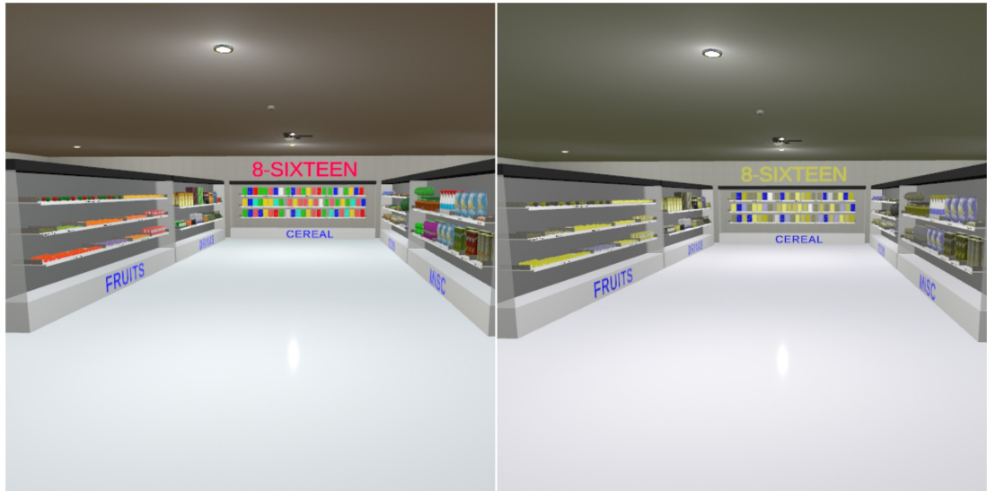
Figure 11. Comparison of the store environment without the CVD filter(left) and with the filter(right).
