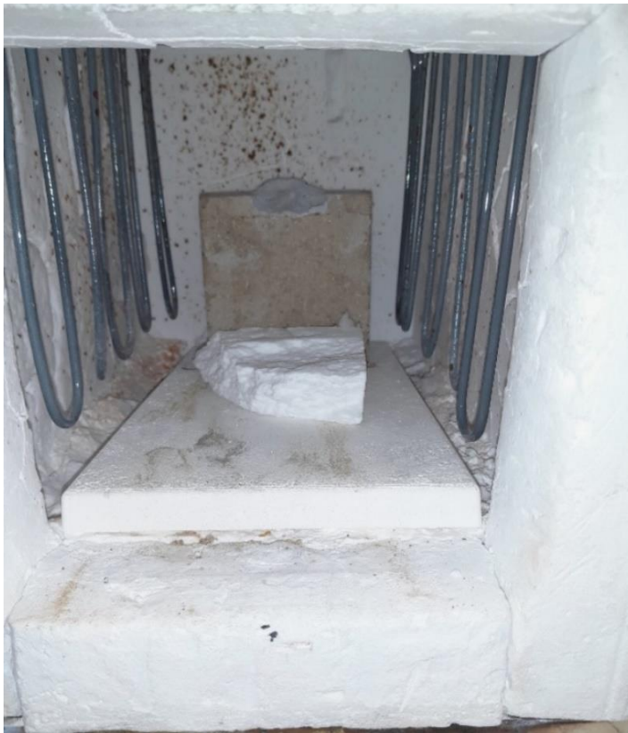
Figure 19. A crucible charged with steel and slag inside the chamber furnace.
