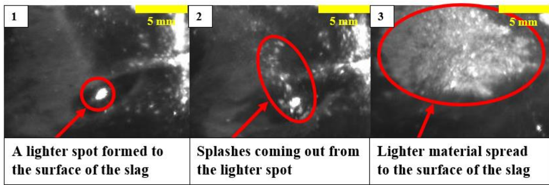
Figure 26. The formation of lighter spots on the surface of the slag during the foaming.
