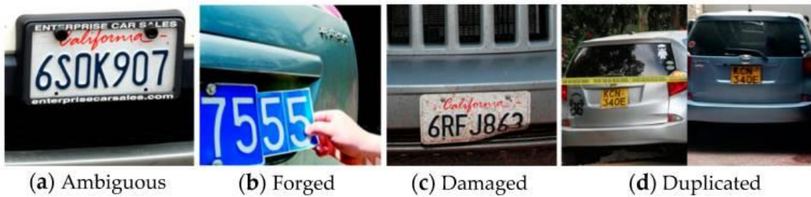
Figure 1: Cases in which LPR algorithms fail [1]
