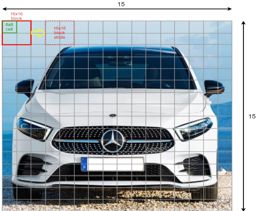
Figure 4: Blocks size, Stride size and scanning positions given the numbers described.
