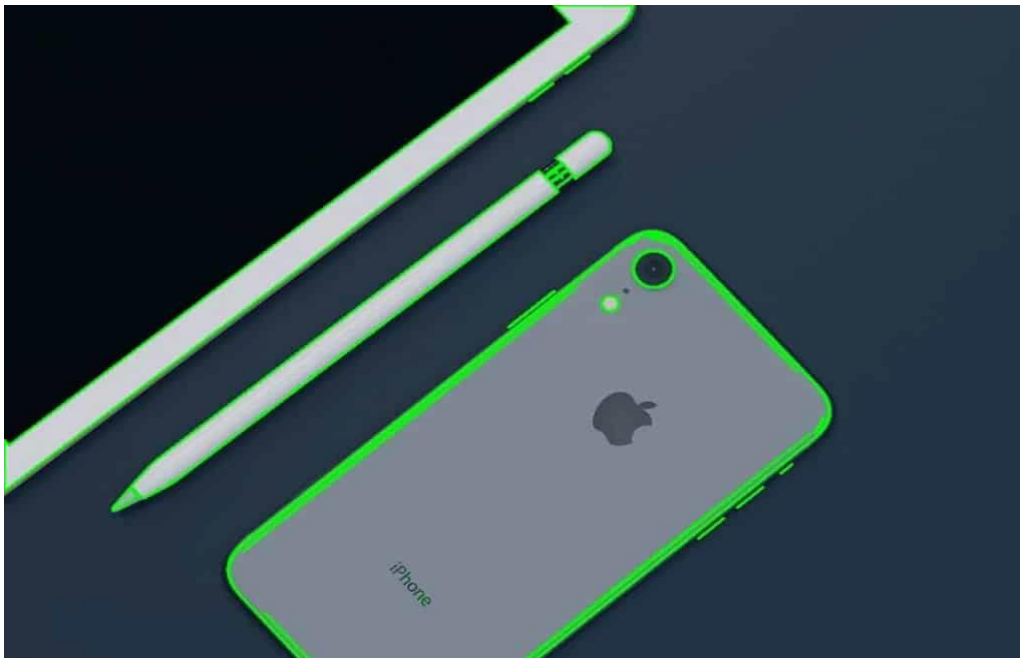
Figure 6: Contours detected using CHAIN_APPROX_SIMPLE method. [17]
