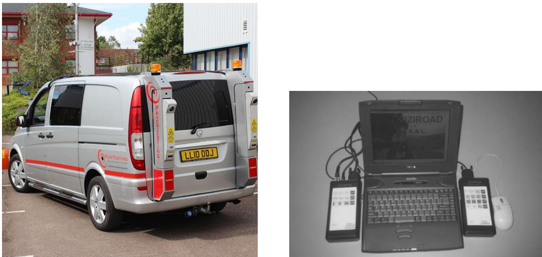
(a) Pavetesting ® lasers installation in a monitoring vehicle. (b) VIZIROAD ® system with 2 keyboards for data acquisition. In this solution, the pavement information is inserted by an operator based on visual observations of the road (Adapted from Picado Santos et al. (2006)).
