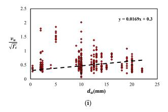
**Figure 1.** Factors influencing the shear strength of steel fiber reinforced (steel fiber reinforced concrete (SFRC)) concrete beam: (a) Concrete compressive strength, (b) Reinforcement ratio, (c) Effective depth, (d) Span to depth ratio, (e) Fiber volume fraction, (f) Fiber factor, (g) Fiber diameter, (h) Tensile strength of fiber, (i) Diameter of aggregate.
