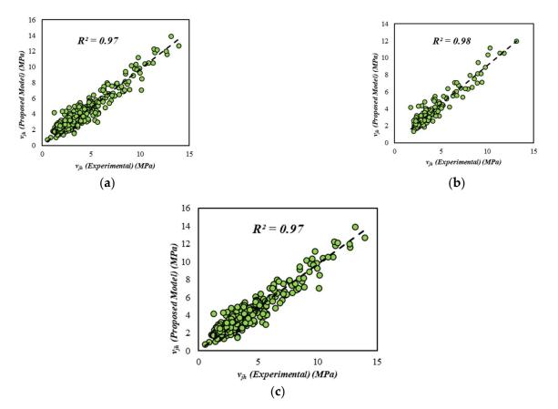
Figure 5. Comparison of estimated and experimental shear strength: (a) Training data, (b) Validation data, (c) All data.
