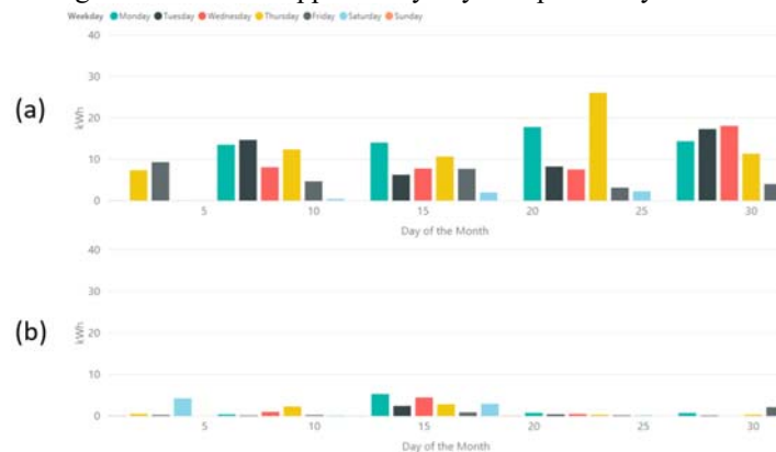
Fig. 7. The daily difference in wasted power between the evaluated auditorium with out-of-reach light switches (a) and one with user-moderated switches (b).
