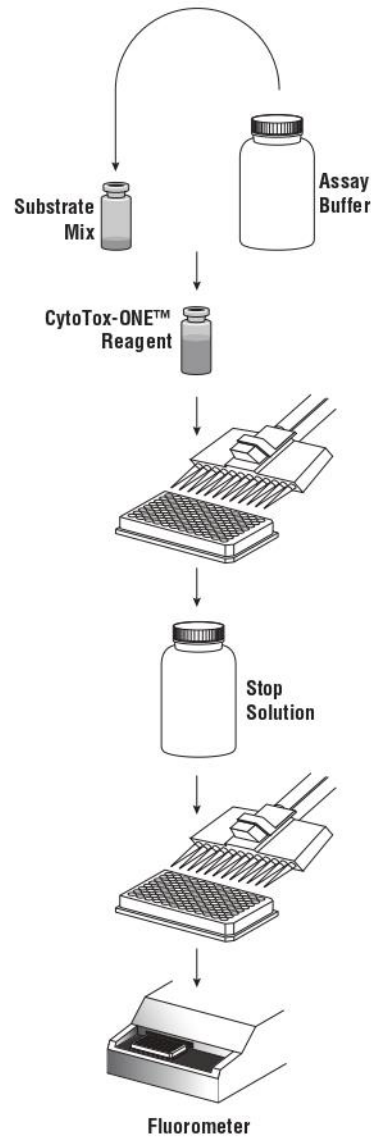
Figure 2. The CytoTox-ONE™ Membrane Integrity Assay protocol. Assay plates are allowed to equilibrate to ambient temperature, and CytoTox-ONE™ Reagent is added to each well and incubated for 10 minutes. Stop Solution is added, and the fluorescent signal is measured.
