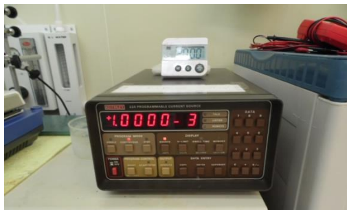
Figure 64 - Current source used in the electrodeposition process (Keithley 220 Programmable Current Source)
