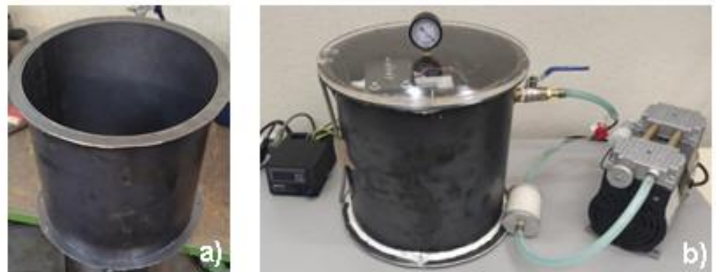
Figure 3. Fabrication and assembly of the Multifunctional vacuum chamber: (a) Welding support rings on the MVC body and (b) Complete set of vacuum chamber and accessories.
