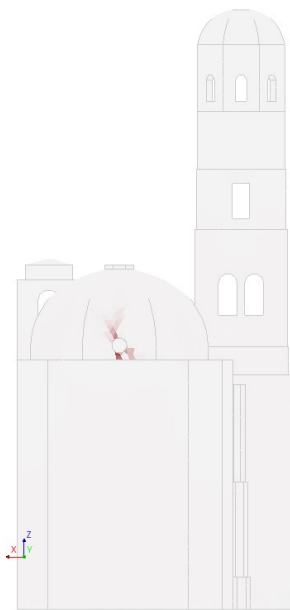
East Elevation. Principal strains E1
