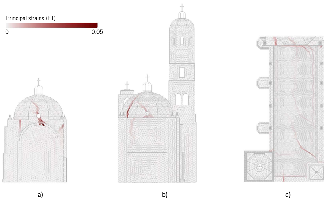
Figure 5-7. Damage in the building due to the action of the signal OXCU: a) transverse arch and dome (section-elevation); b) back wall (elevation); c) extrados barrel vault (plan).
