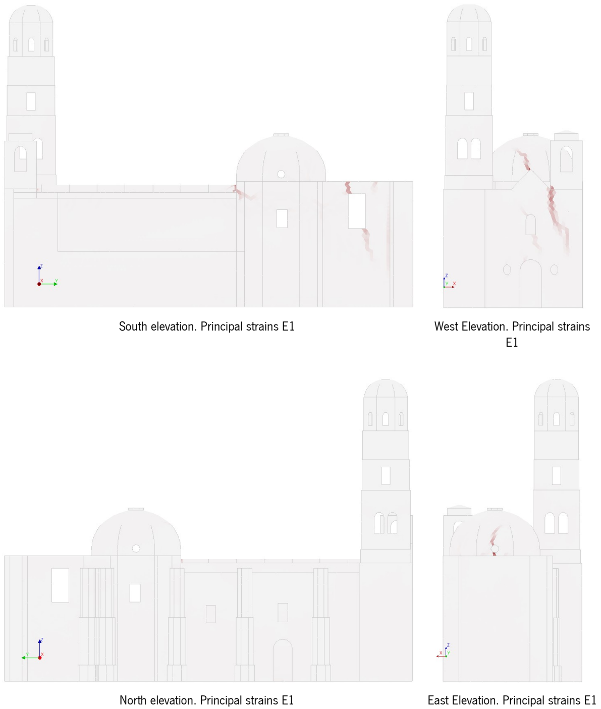
Figure C - 18. Post-peak damage state caused by the Pushover analysis +X.
