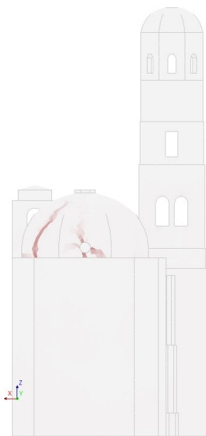
East Elevation. Principal strains E1
