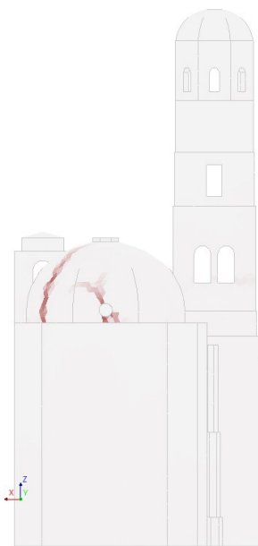
East Elevation. Principal strains E1
