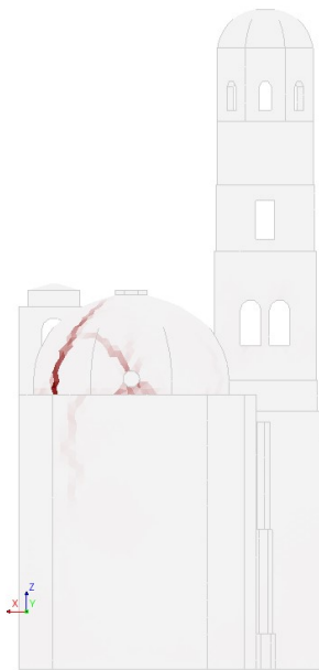
East Elevation. Principal strains E1
