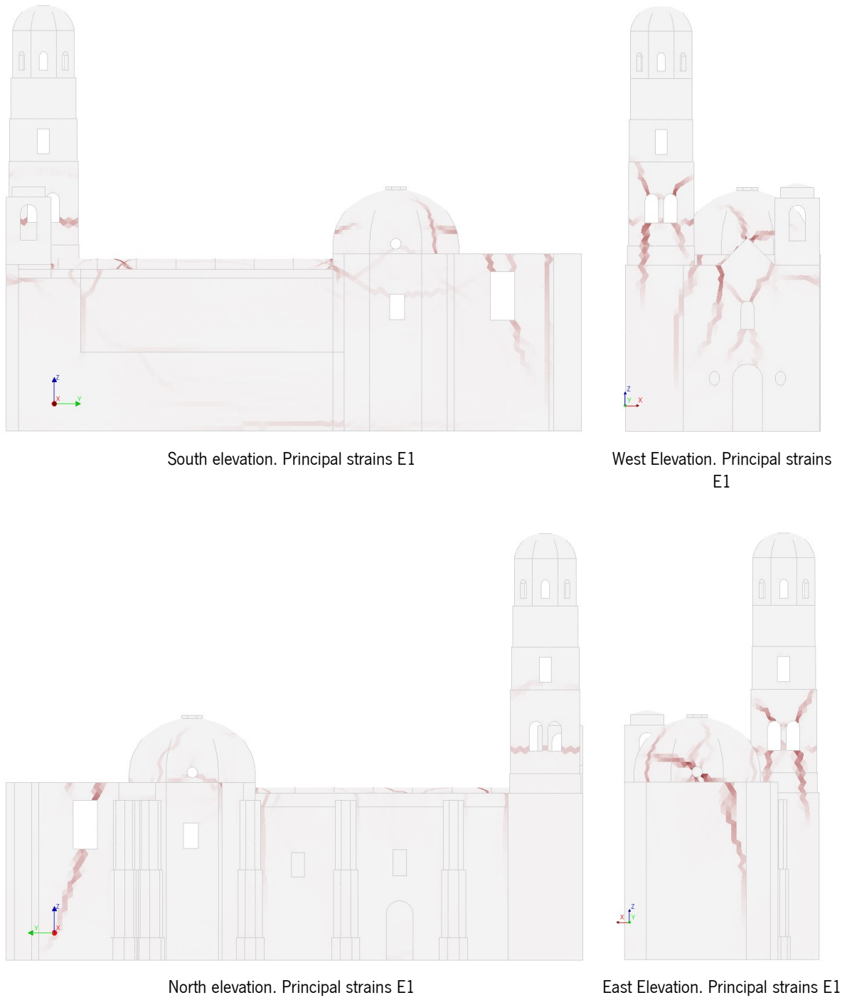
Figure C - 16. Damage caused by the THEZ record.
