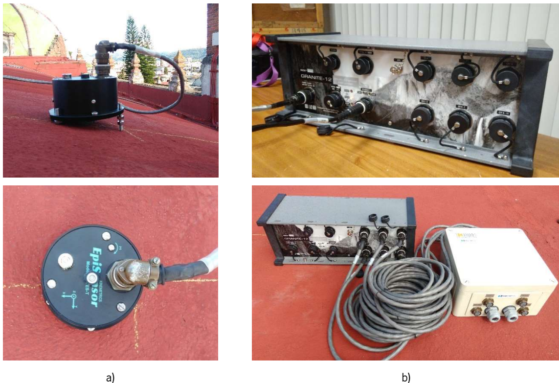
Figure 4-10. Equipment used in the dynamic identification tests: a) Force Balance Accelerometer; and b) Communication Centric Multi-Channel Recorder.
