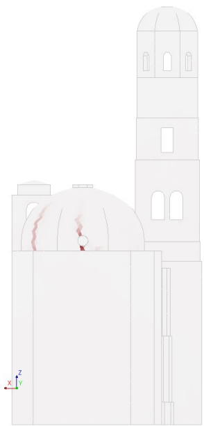
East Elevation. Principal strains E1
