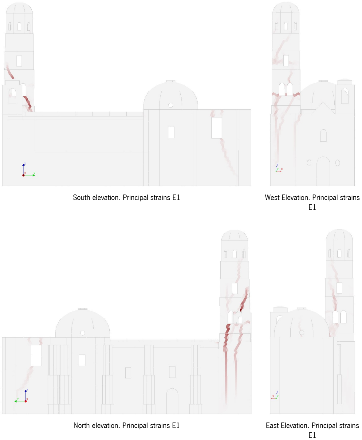
Figure C - 22. Post-peak damage state caused by the pushover analysis +Y.
