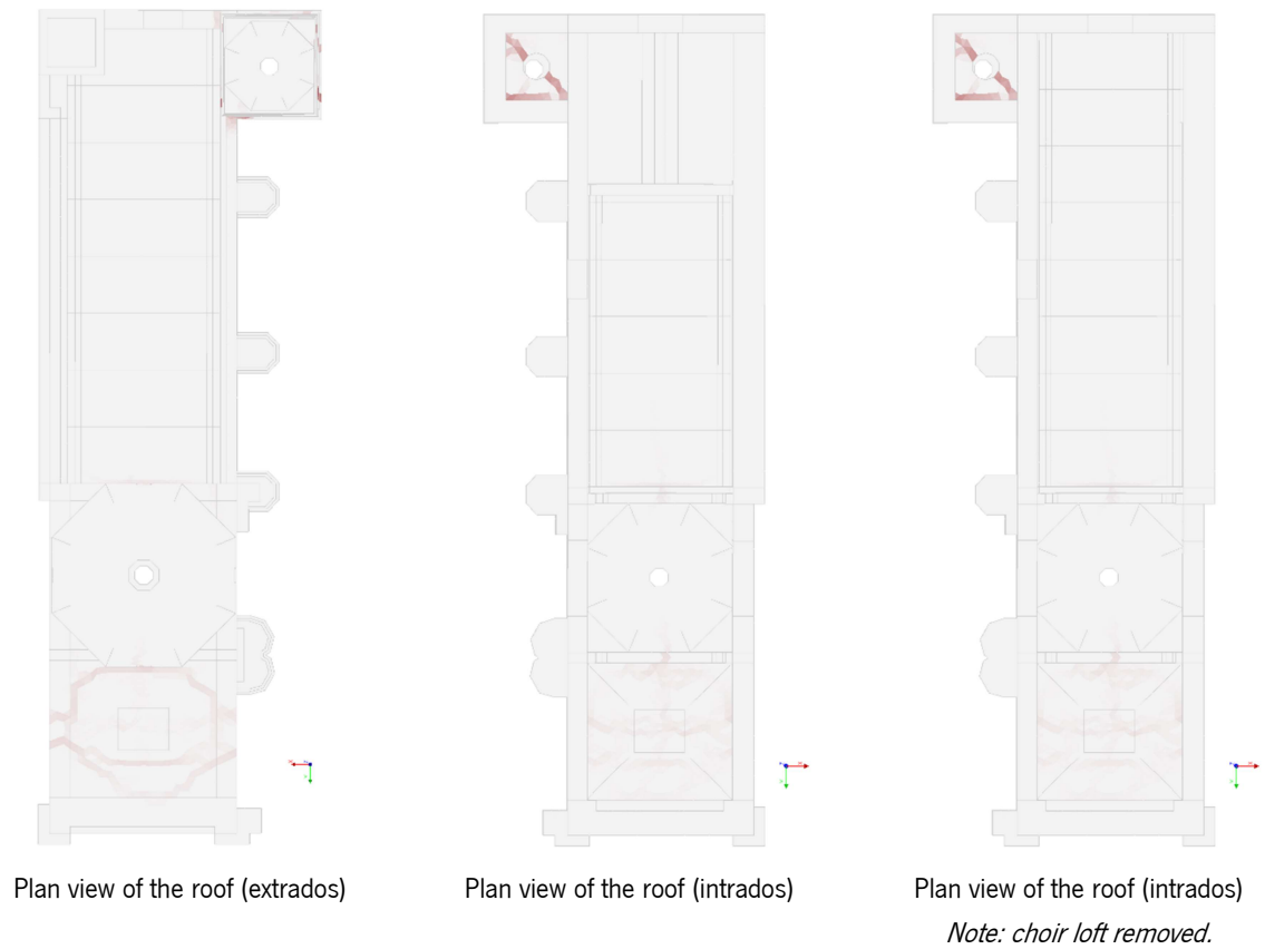
Figure C - 21. Post-peak damage state caused by the pushover analysis +Y.
