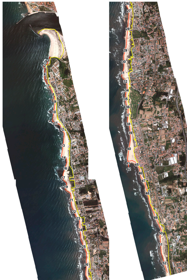
Figure 8. Orthomosaic of the aerial photographs, with the analysed coastal segments (simplified 1 m isoline in red, segments labelled with their ID numbers) and the delimitation of the beach-dune system (yellow line); segment 14 marks the Canide groyne, segments 41 and 42 mark the Aguda breakwater.
