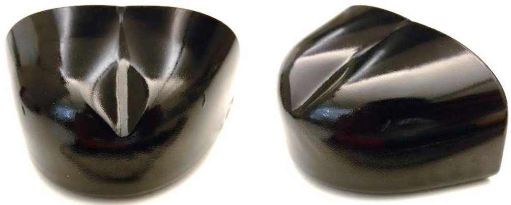
Figure 21. Geometry of a toe cap subjected to the impact test.
