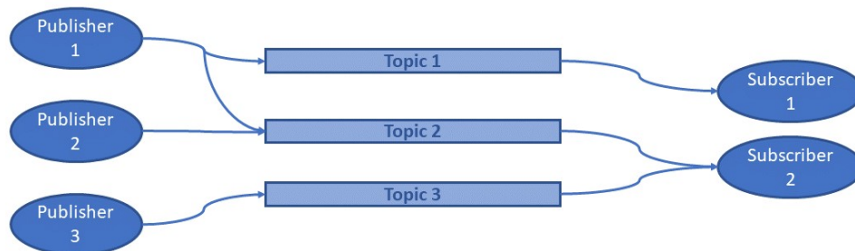
Figure 3: Communication structure of Robot Operating System.
