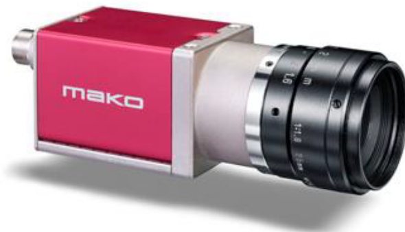
Figure 42: Illustrative image of the Allied Vision MAKO G-234c camera. 1
