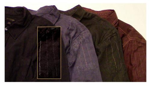
Figure 2: Ripple shirts have embedded skin conductance sensors. They display spikes in skin conductance, a loose proxy for various kinds of excitement, with three embroidered thermochromic pinstripes that gradually change, one by one, between dark gray and white.
