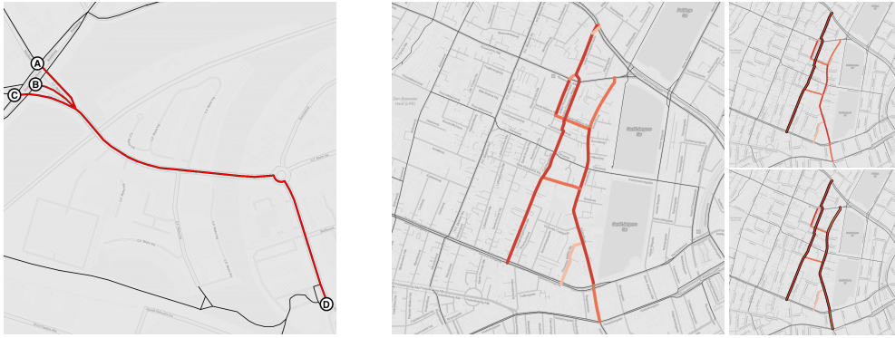
FIGURE 6 Example of gap clusters, and of the declustering heuristic. Left: Shown in red, on C.F. Richs Vej. The three gaps AD, BD and CD overlap and have similar closure benefits B(g) . Therefore, the three gaps are merged into one gap cluster to be handled jointly. Right: A declustering heuristic can help deciding which parts to retain and which ones to discard. The links of the shown gap cluster are colored by betweenness centrality; darker tones represent higher values. The black borders indicate the declustered gaps after one and two runs of the heuristic.
