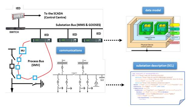
Figure 1: Elements of the IED 61850 standard.
