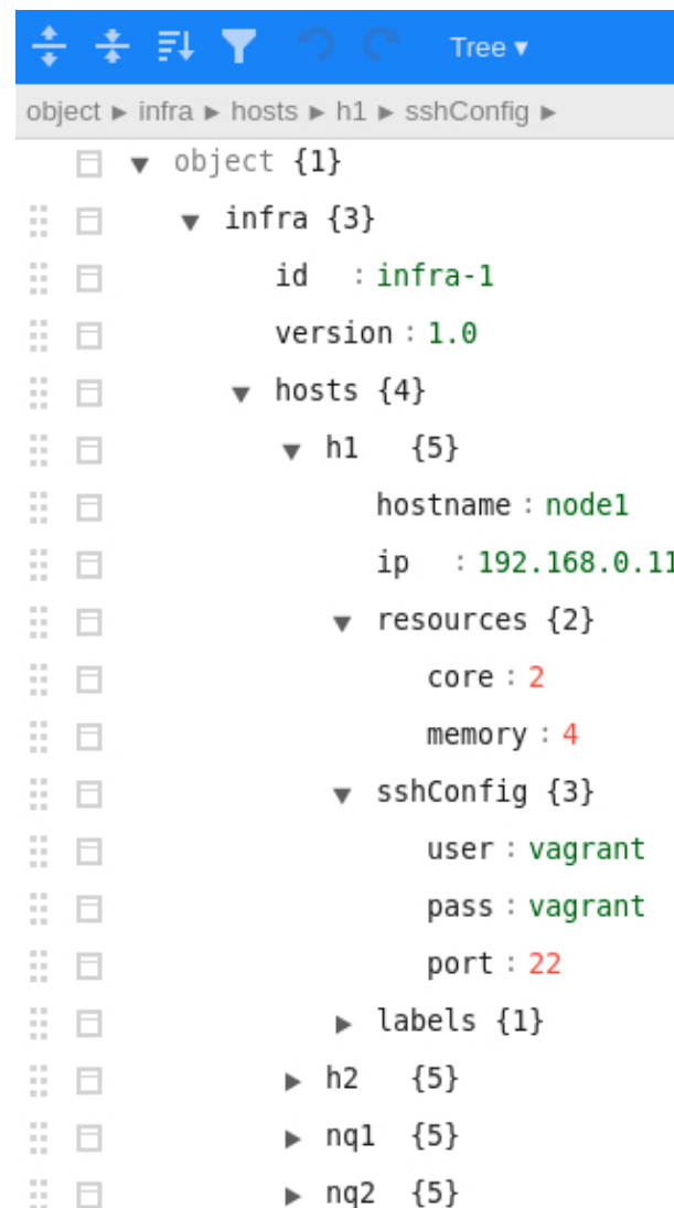
Figure 11. Screenshot of the client when editing the infrastructure definition. An example of the required properties of each node is represented.
